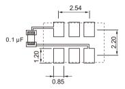
To ensure optimal oscillator performance, place a by-pass capacitor of 0.1  $\mu\text{F}$  as close to the part as possible between Vdd and GND pads.
