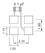
To ensure optimal oscillator performance, place a by-pass capacitor of 0.1  $\mu F$  as close to the part as possible between Vdd and GND pads.
